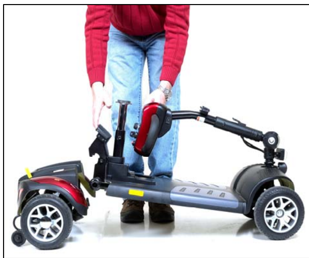
Figure 20. Connecting Frame and Drivetrain
