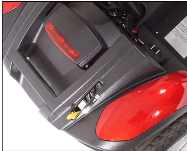
Figure 11: Freewheel Lever (Drive Position)
