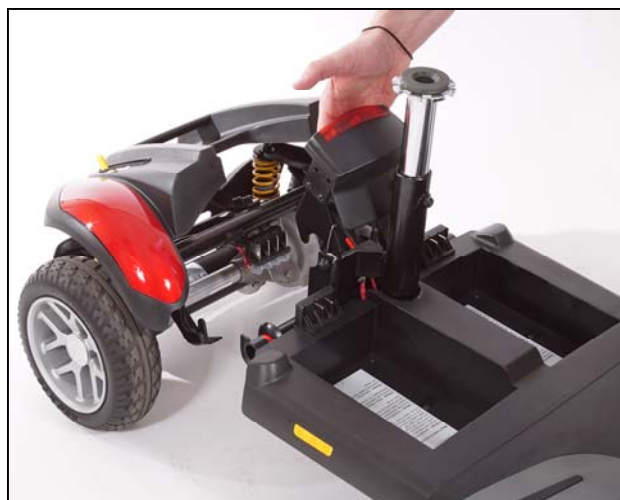
Figure 17. Separating the Drivetrain and Frame
