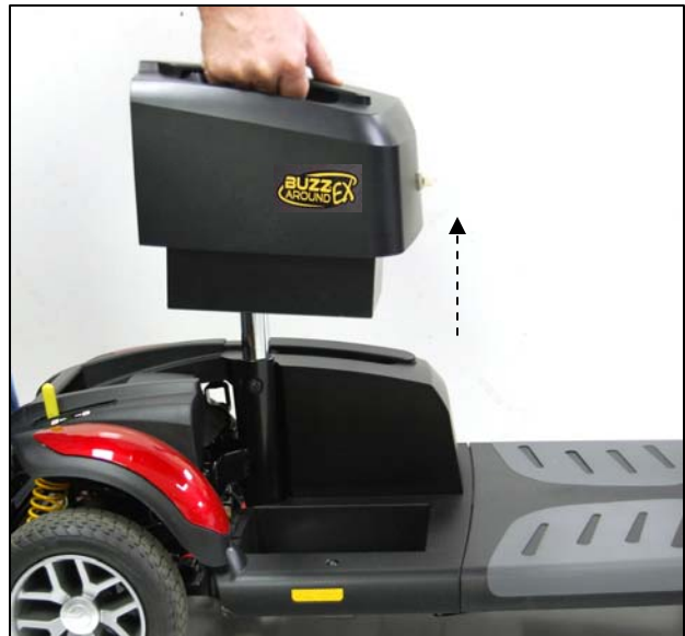
Figure 15. Removing the Battery Pack
