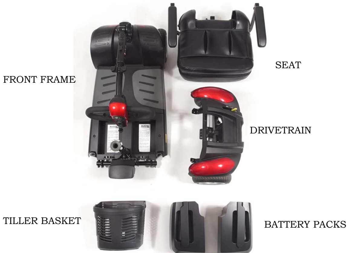
Figure 18. Buzzaround Extreme™ Components (Model GB148EX)
