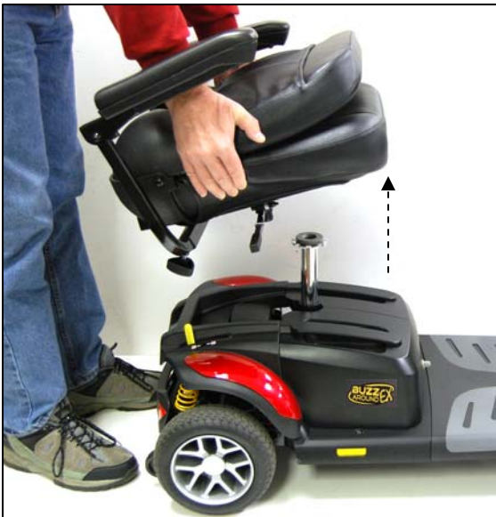
Figure 14. Removing the Seat
