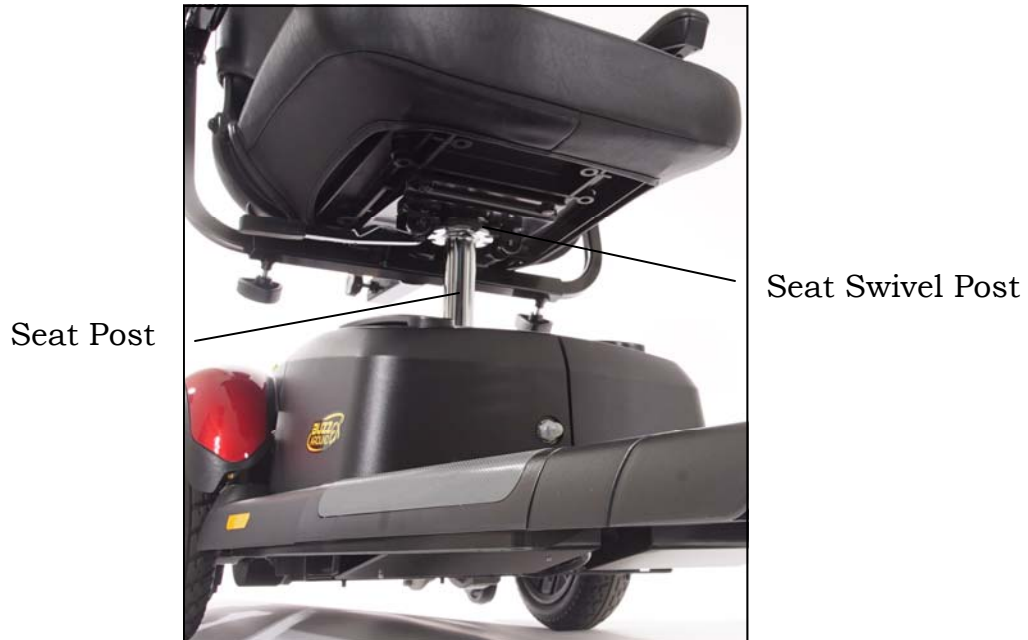
Figure 23. Installing the Seat
